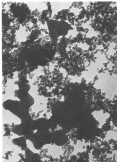
Figure 5. Sample 1 in Table II calcined at 1000°C \theta - and \alpha -aluminas; magnification, \times 50,000
